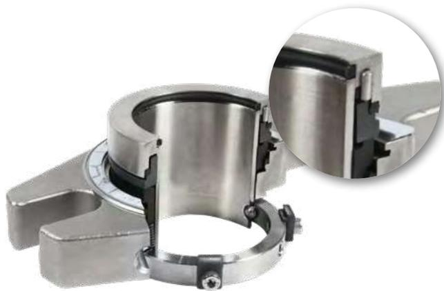
•The springs for compressing the contact surfaces are isolated from the product, which prevents them from becoming blocked by products containing particles, pastes, etc. They are made of Hastelloy material and have great chemical resistance and mechanical properties superior to those of stainless steel.
