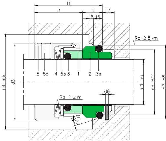
Tolerancia l, d, 14...25 mm ± 1.0; 28...63 mm ± 1.5; > 65 mm ± 2.0
